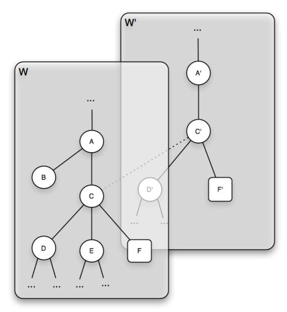
The above diagram depicts two workspaces W and W'. Node C in W and node C' in W' are corresponding nodes. Note that the subgraphs of corresponding nodes may differ, as they do in this case.
