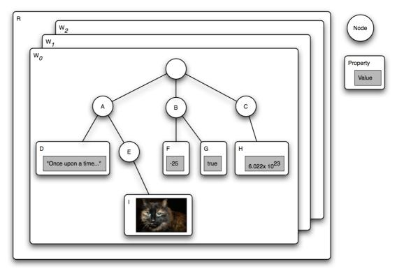
The above diagram depicts a repository R with workspaces  $W_0$ , W1 and  $W_2$ . The item graph of  $W_1$  contains a root node with child nodes A, B and C. A has a property D of type STRING and a child node E, which in turn has a property I of type BINARY. B has the properties F (a LONG) and G (a BOOLEAN). C has a property H of type DOUBLE.
