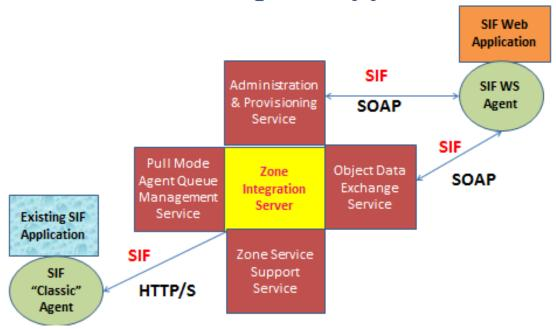
Figure 1: Example of the SIF Infrastructure Web Service (SIWS) seamlessly supporting exchanges between a SIF web application over SOAP, and a SIF agent/application component over the alternate HTTPS transport.
