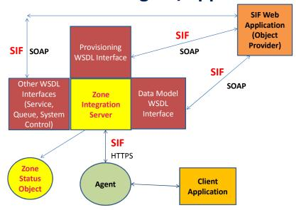
Figure 1: Example of the SIF Infrastructure Web Service(SIWS) transparently and simultaneously supportingboth a "Pull Mode" SIF Web Application (SWA)over SOAP, and an "original" SIF Agent / Application component over the original HTTPS transport.
