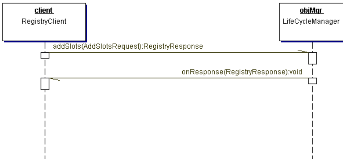
Figure 9: Add Slots Sequence Diagram
