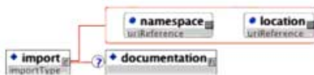
Figure 2.3 <import> element structure.
