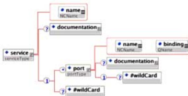
Figure 2.8 <service> element structure.
