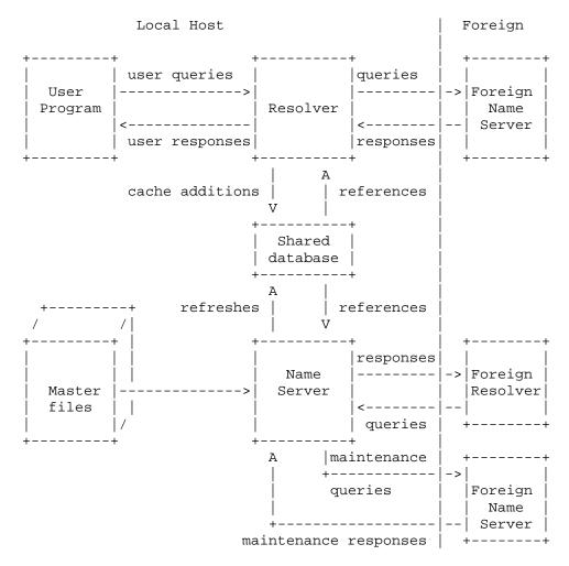
The shared database holds domain space data for the local name server and resolver. The contents of the shared database will typically be a mixture of authoritative data maintained by the periodic refresh operations of the name server and cached data from previous resolver requests. The structure of the domain data and the necessity for synchronization between name servers and resolvers imply the general characteristics of this database, but the actual format is up to the local implementor.
