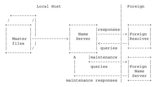
In this configuration, the name server periodically establishes a virtual circuit to a foreign name server to acquire a copy of a zone or to check that an existing copy has not changed. The messages sent for
