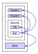
Note: if required, the initiator may also include in the Security header the token used as the basis for the message signature (Sig1), not shown in the diagram.
