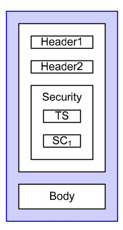
The blue outer box shows that the entire message is protected (signed and encrypted) by the transport. One <code>wssell:SignatureConfirmation</code> element labeled  $SC_1$  corresponding to the signature in the initial message illustrated previously is included. In general, the ordering of the items in the security header follows the most optimal layout for a receiver to process its contents.
