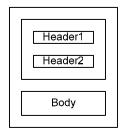
Each binding requires that the message is signed using a token satisfying the required usage for that binding, and that the signature (Sig1) covers important parts of the message including the message timestamp (TS) facilitate replay detection. The signature is then included as part of the Security header as illustrated below:
