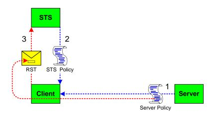
Before the Client sends the RST to the STS, it will need to obtain the policy for the STS. This will help to formulate the RST request and will include any security-specific requirements of the STS.
