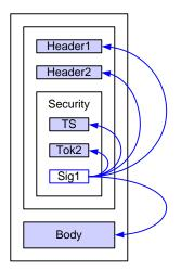
If transport security is used, the token (Tok2) is included in the Security header as illustrated below:
