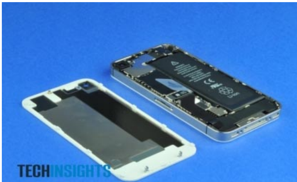
The back cover of the iPhone 4S removed reveals the main board and the battery.
