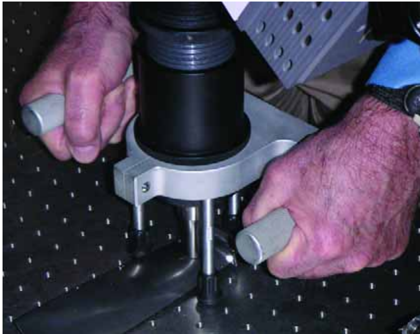
Injecting ultrasound into an aircraft engine turbine blade with a handheld ultrasonic gun. Photo courtesy of Skip Favro, Ph.D., Wayne State University
